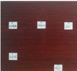
Lacper® 4703优异的耐化学品性能 Lacper® 4703 excellent chemical resistance
